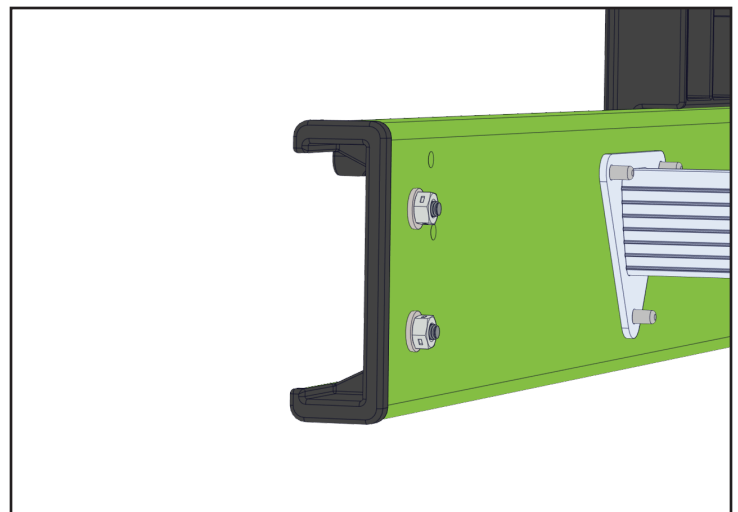
12. Make sure end cap and any accessories are tightly secured before use.
